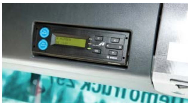
Figure 1 On-Board Unit for satellite-based vehicle log-in to the truck toll system
